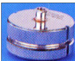
A re-usable **Stainless Steel Holder** for particle removal and sterilisation of up to 100ml volumes of solvents and aggressive liquids. Filter supports in the top and bottom parts allow filtration in either direction. No sealing ring or gasket is required, as a PTFE coated surface on the top part ensures leakproof sealing using the tightening tool in which the holder is supplied. The holder can be sterilised by auto-claving or in an oven at 180°C.
