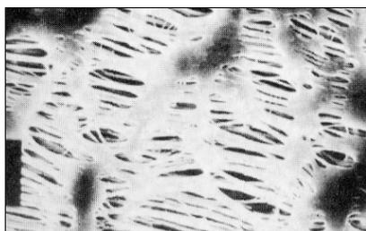
Type 118 **hydrophobic** membranes for the filtration of **air, gases** and **chemicals**.
