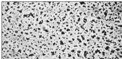
Membranes with high flow rates, very low adsorption characteristics coupled with thermal stability. This makes the 0.2µm pore size excellently suited for use in disc filter holders to sterilise aqueous solutions, buffers, sera and media.
