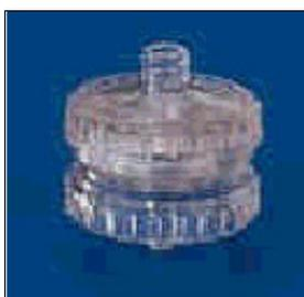
This inexpensive, re-usable holder is made of clear, autoclavable poly-carbonate and contains a silicone gasket for leakproof sealing. It can be used at pressures of up to 7 bar. Filter supports in the top and bottom parts allow filtration in either direction. The milled edges make hand tightening easy.
