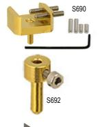
Rectangular type bulk sample holder with pin (or M4) and two side brackets for sample thickness up to 16mm. Made from brass,  $1\mu m$  thick gold plated. Ideal for smaller samples and smaller SEMs. Provided with 4 set screws.
