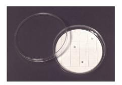
Silicone rubber indexed grid storage and transport plate housed in a polystyrene Petri dish. The ideal way of storing 'working' grids. The grids adhere lightly to the surface of the silicone mould, which eliminates the problem of grids jumping. The grids when required are easily picked up with tweezers. The grid disc are also available separately should you wish to supply your own plastic or glass Petri dishes. Available in sizes to fit 90mm or 50mm diameter Petri dishes.
