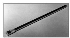
Nickel-plated brass, holder is fitted with screw chuck. Suitable for wire or needles up to 0.056mm diameter (24 SWG). Overall length of holder is 150mm
